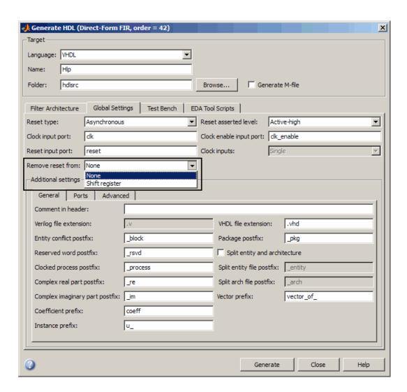
You can also use generatehd1 function with the property RemoveResetFrom to suppress generation of resets from shift registers.
