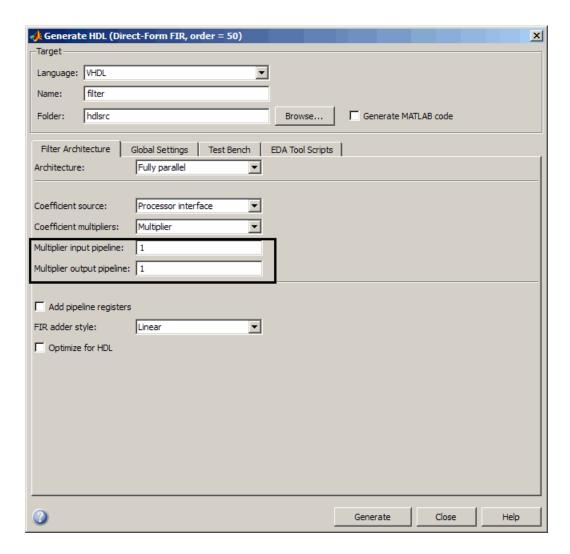
The coder enables the **Multiplier input pipeline** and **Multiplier output pipeline** options when **Coefficient multipliers** is set to Multiplier.
