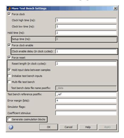
Each new option (except **Setup time (ns)**) has a corresponding command-line property. The following table lists the new options and their corresponding command-line properties, and provides hyperlinks to the relevant documentation.
